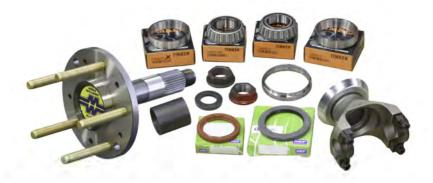
50230-KIT• C2-C3 Corvette Next-Step Rear Axle-Yoke Assembly • Replaces the weak 17-spline axles with 31-spline, and a one-piece u-Joint flange yoke.
