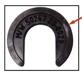
M/W offers an extra thick hardened C-Clip, P/N 50247. This C-Clip can be machined to the precise thickness needed. The basic thickness is .180" and can be machined down to .140". Note: the stepped side of the washer goes against the axle gear.
