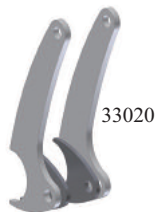
15010 Axle Mount Brackets F/C (4) . . . . .61.00 3/16 4130 welds to 1-5/8" tube axle bolts to the 35000 Torsion
