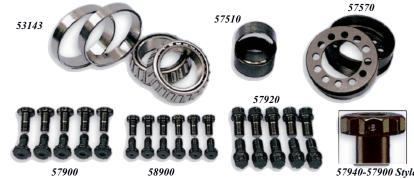
All MW spool bearing kits feature Timken® bearings and races. MW also offers special bearing adapters to allow the use of spools for smaller bore sizes to be used in larger bores. MW ring gear bolts are manufactured with a ground shoulder to drive against, while the 12 point bolt heads are drilled to accept aircraft type safety wire. This method reduces the chance of the ring gear bolts "backing out".
