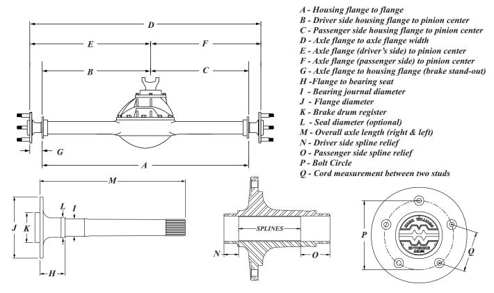
**STARTING FROM SCRATCH** The following steps have proven to be the most accurate method for determining the width of the rear end assembly when building a new car.
