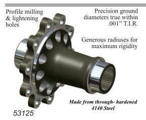
There is more to a spool than meets the eye. It not just a pretty part, but one of the key components that influence ring and pinion life. Our product has a reliable ratio of strength to weight. MW steel and aluminum spools are in-house produced from our exclusive forging tools that create superior grain flow for maximum strength. MW steel spools are produced from 4140 alloys and through hardened, resulting in steel strength that is the same at the core as at the surface.
