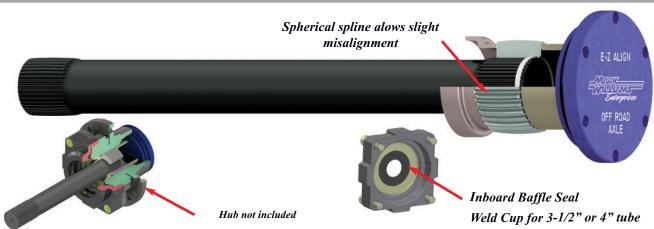
The F350 Unit hub is an economical and bulletproof way to upgrade from a conventional truck floater. MW offers axles with the Donut Spline Adapter and cover that are made to fit the OEM hub. Our EZ-Align splines are manufactured with a slight crown that allows some misalignment without bowing the axle shaft. This bowing creates forces on the housing's center section that will eventually destroy gears and bearings.
