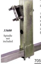
The MW A-Arm jig simplifies installing an aarm front end on a dragster or funny car chassis. The spindle is fastened through the upright and set to the proper caster angle with a bubble protractor. This is normally used for cars with standard 17" dragster or 15" FC spindle mount front wheels. The uprights can be positioned anywhere along the 1-1/2" square cross tube (included) to produce the desired front end
