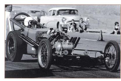
By 1960, Williams had built his first dragster. Based on an article in an East Coast rodding magazine, it was built from old driveshafts and powered by an injected Oldsmobile. He says, "At the time, I didn't really know how to weld, but that didn't stop me."
