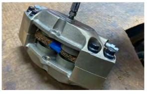
2) With shop air inflate the brake fluid chamber to push the pistons against the shim. It takes very little pressure to move the pistons.
