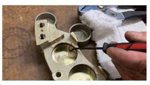
5) Remove the piston and fluid passage o-rings with a hook pick tool. Be careful not to scratch or mar the sidewalls of the o-ring groove
