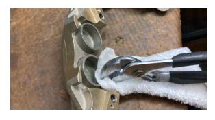
4) Gently with a channel lock pliers (jaws cushioned) remove each piston. Be careful not to mar the piston.
