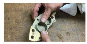
7) When cleaned, reassemble by soaking the o-ring in brake fluid to make the insertion of the piston easier. Gently push the pistons in the caliper halves. Do not force the piston as it can shear the o-rings and cause leakage.
