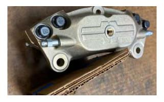
1) Remove both brake pads. Place a shim, like the cardboard shown above, in the slot from the bottom that extends over the bottom mounting lugs and covers the piston areas. This example used 3 pieces of cardboard for the shim.
