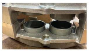
3) The pistons now stick out almost past the o-ring seals. Disassemble the caliper by removing the 5/16" bridge bolt and spacer and the 4 ea 7/16" reduced hex fasteners. <u>Caution</u>: The brake fluid remaining in the caliper will be free to leak out.
