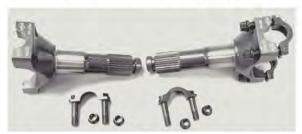
50248-KIT • C2-C3 Rear Inner Yoke Shafts for modified C2-C3 Differentials for rears that have the Tom's Gears modified 12 bolt carrier and special ring and pinion gears.
