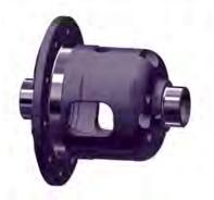
ACG-030 • C2-C3 Replacement Case for the Eaton™ 19670 Positraction • The is Case produced from thru-hardened alloy steel that solves the problem with cracked and failed cases while increasing gear life. It use 12 Bolt GM axle side and pinion gears for the 30 spline inner shafts.
