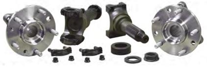
50225-KIT • C4 '88-'96 Corvette Rear Hub and Yoke Shaft Kit • Features new Timken™ hubs with a larger 32-spline and matching 300M Yoke with Billet Caps.
