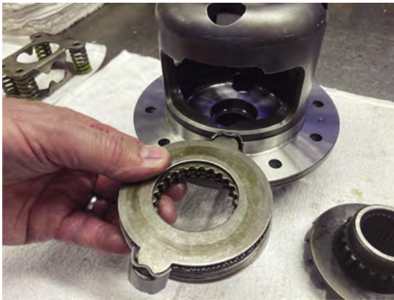
The first clutch pack is installed in the ring gear side of the case. This sequence must be followed to get everything to go in.
