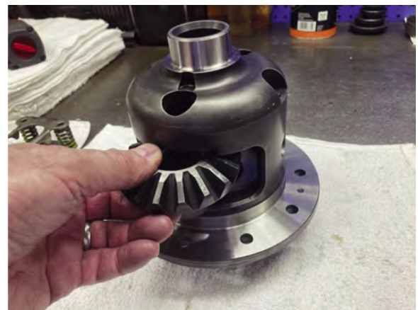
The first axle gear is installed and dropped into the clutch pack.
