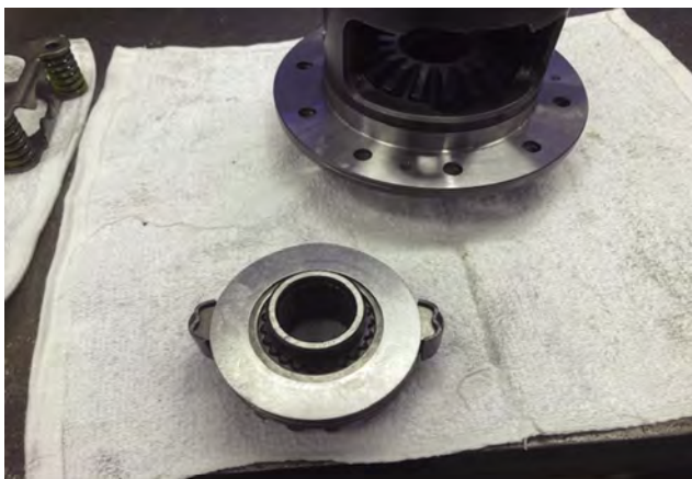
The second clutch pack is placed on the axle gear to align the floater plates.
