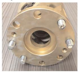
8) Install two drive studs (MWS-670) into the transmission flange on the vehicle using a 7mm hex wrench and torque to 30-35 ft\*lbs. Use (Loctite red threadlocker 271). The studs must be clocked in the flange as shown in the picture below to ensure the correct alignment into the blind holes of the driveshaft u-joint flange. Note this photo only shows the stud clocking it does not show the studs installed into the transmission flange.
