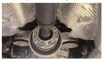
5) Now remove the six torx head bolts on the transmission side CV flange, using a T50 torx bit and separate the front of the driveshaft from the transmission.
