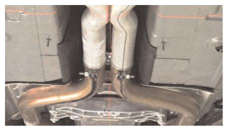
2) After the rear exhaust system has been removed unbolt and remove the heat shield.
