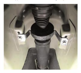
**4)** Next remove seven of the eight torx head bolts on the differential side CV flange using a T50 torx bit. Leave one of the bolts engaged into the thread to support the driveshaft during step 5.
