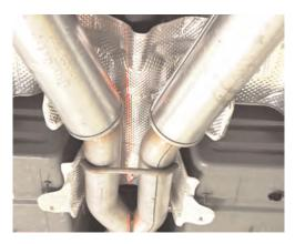
3) Now loosen the two bolts that hold the center carrier bearing to the vehicle using a 13mm socket. Leave one of the bolts engaged into the thread to support the driveshaft during steps 4 & 5.
